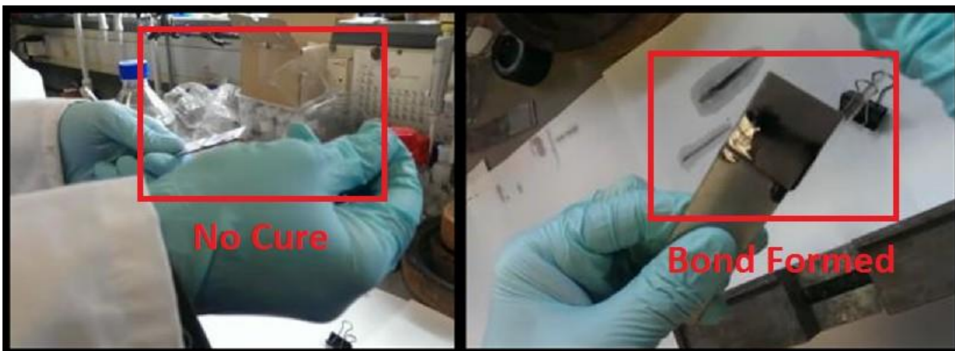
Acrylic formulation tested on SS to glass. Bond is formed only when exposed to magnet
